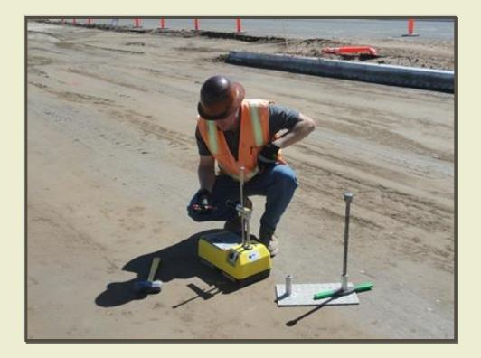
Use conventional testing methods such as nuclear gauge and sandcone methods
